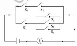
(where p, q and r represents switches s<sub>1</sub>, s<sub>2</sub> and s<sub>3</sub> which are closed respectively)
